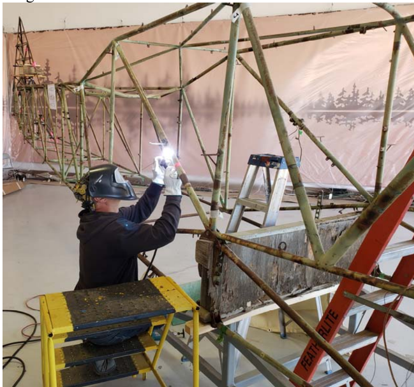
Welding a new shelf bracket in place
